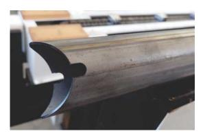
Max tube lenght: 6000mm Max tube diameter: 250mm Laser power: 3000W
