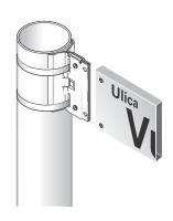
Signs are made of Aluminium profile mounted with Strap clamp
