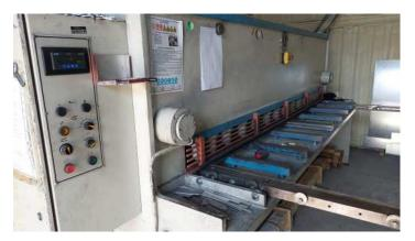
Hidraulic press for cutting metal sheet plates
