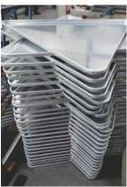
Bending edges is done around the whole sign base plate, without cease
