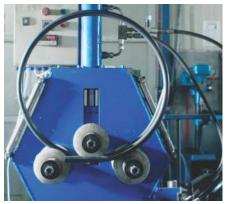
Machine for tube bending. Max tube diameter: 3/4" - 2.5"
