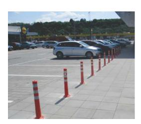
Flexible plastic pole, height: 750mm
