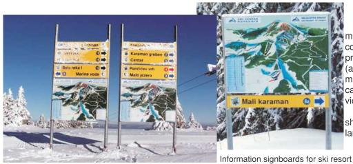
Information boards are manufactured, as required, out of a combination of materials including Al profiles, Al sheets, steel pipes, klirit (acrylic glass). Information boards may contain illuminated elements in case of a power supply source in the vicinity.
