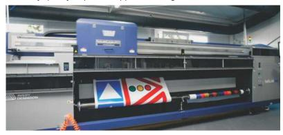
UV LED large roll to roll printer (3m max. print width) provided by **AVERY** is high production machine capable of printing on 2 roll of sheeting (1,23 m, standard width of reflective sheeting roll) in a same time. Print can be done on various material from commercial program: PVC sheeting, tarpaulin, Blue back paper, One Way Vision...
